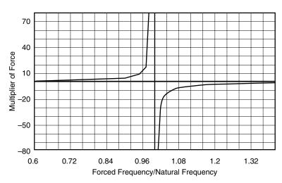
FIGURE 10.1 Natural versus forced frequency
