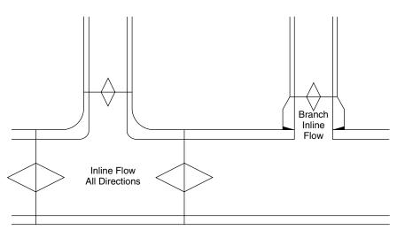
FIGURE 6.6 Schematic of inline and branch outlet differences
