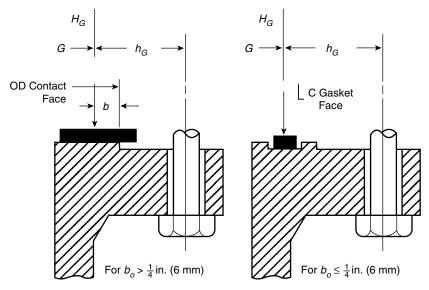
FIGURE 6.7 Gasket reaction diameter
