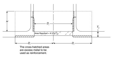
FIGURE 6.5 Generic extrusion area replacement
