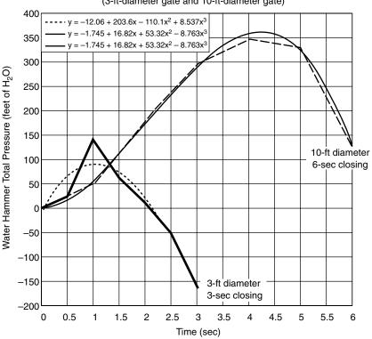
Total Water Hammer Pressure versus Time (3-ft-diameter gate and 10-ft-diameter gate)
