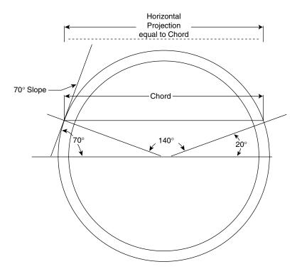
FIGURE 11.8 Horizontal width of pipe for snow loads
