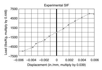
FIGURE 7.6 Example load/unload SIF chart
