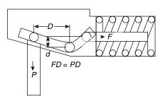
There can be a situation where one cannot find a standard spring hammer, or for one reason or another, variability of the load has to be tighter than the 25 percent or even the 10 percent criterion mentioned for critical systems. In those cases a constant force–type support is required. While there are some standards, according to MSS they are generally in the 6 percent variability range. Anything more critical would most likely be special.
