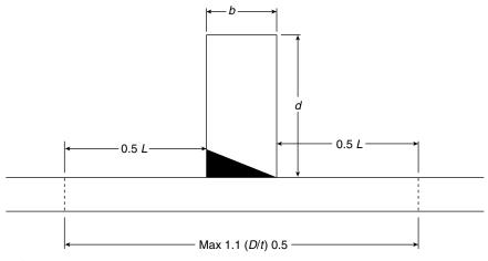
FIGURE 5.4 External pressure stiffener example
