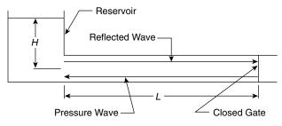
FIGURE 12.1 Water hammer diagram
