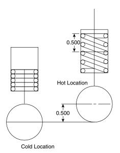
FIGURE 8.3 Spring hanger hot and cold positions
