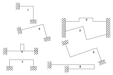
FIGURE 7.2 Common piping shapes
