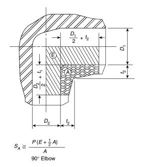
FIGURE 6.4 Pressure area elbow
