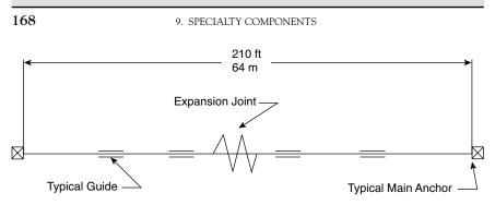
FIGURE 9.2 Expansion joint support calculations example
