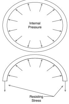
This is the basic equation that the code presents. Since the goal is to find the unknown thickness, the formula is rearranged to solve for *t* given the other three parameters: pressure, outside diameter (OD), and allowable stress. The formula then becomes
