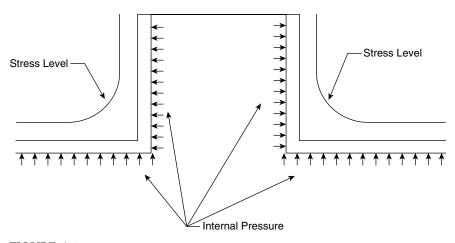
FIGURE 6.1 Intersection stress increase diagram
