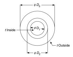
FIGURE 13.1 Pipe with one layer of insulation
