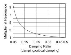
FIGURE 10.2 Multiplier effect of damping ratio
