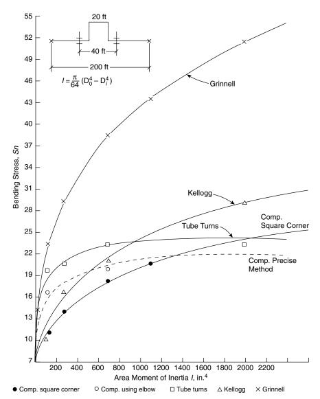
**FIGURE 7.3** Variability of flexibility analysis methods (*Source:* From Kannappan, *Introduction to Pipe Stress Analysis;* used with permission.)
