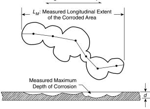
FIGURE 13.3 Typical corrosion spot (*Source:* From ASME, B31-G, figure 2.2; used with permission.)
