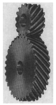
Figure 14-4 Typical set of helical gears (Neale 1993).
