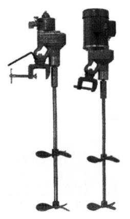
Figure 11–1 Top-entering propeller-type mixer (Thomas Register 1995).
