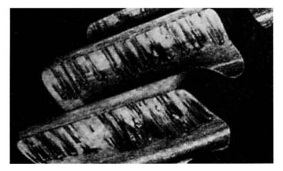
Figure 3–7 Visual profile of badly worn spur gear.
