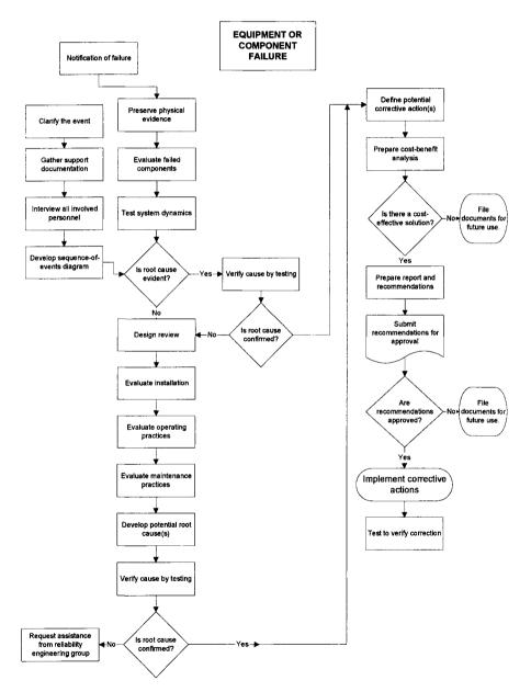
Figure 3-5 Flow diagram for equipment failure investigation.
