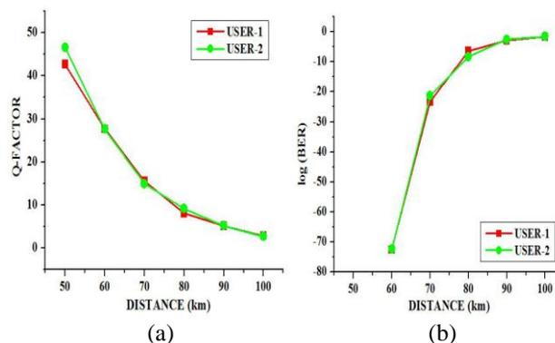
Fig. 8: Relationship of (a) Q-factor and (b) log (BER) with Distance for Bidirectional BPON with 2 users in the Downstream Direction
