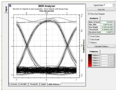
Fig. 9: Eye Diagram for OLT of the Bidirectional BPON at 70km in the Upstream Direction
