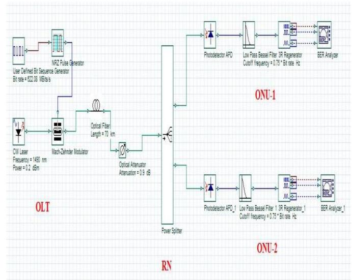
Fig. 2: Simulation Layout of Unidirectional BPON with 2 Users
