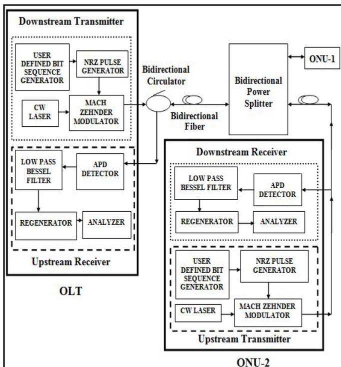
Fig. 3: Block Diagram of Bidirectional BPON with 2 Users
