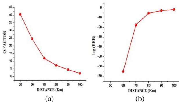
Fig. 10: Relationship of (a) Q-factor and (b) log (BER) with Distance for Bidirectional BPON in the Upstream Direction
