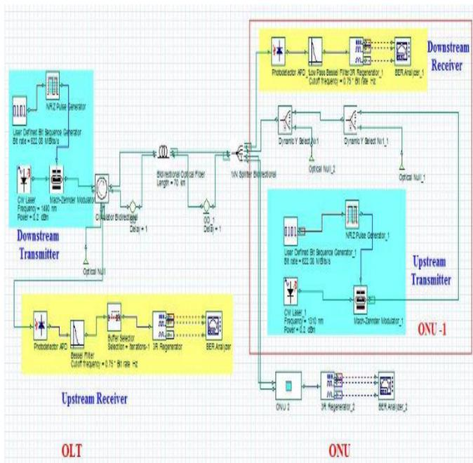
Fig. 4: Simulation Layout of Bidirectional BPON with 2 Users
