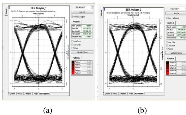
Fig. 7: Eye Diagrams for the (a) First User (b) Second User of the Bidirectional BPON at 70km in the Downstream Direction
