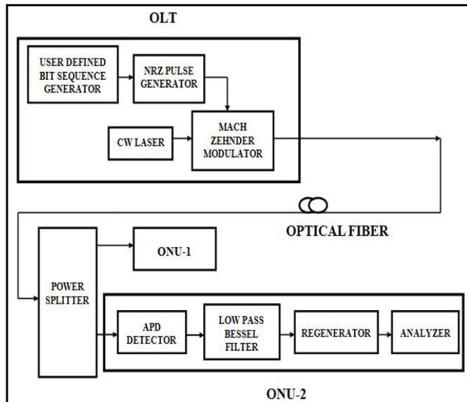
Fig. 1: Block Diagram of Unidirectional BPON with 2 Users
