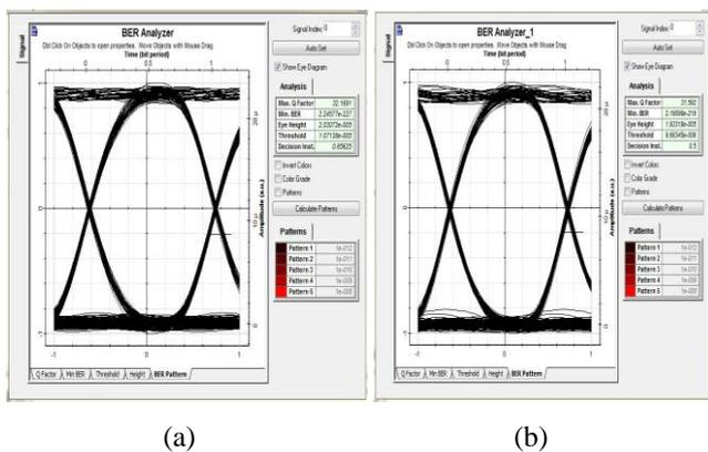
Fig. 5: Eye Diagrams for the (a) First User (b) Second User of the Bidirectional BPON at 70km in the Downstream Direction
