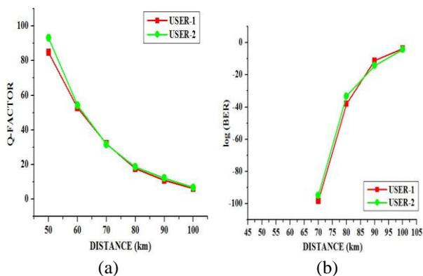
Fig. 6: Relationship of (a) Q-factor and (b) log (BER) with Distance for Unidirectional BPON with 2 users
