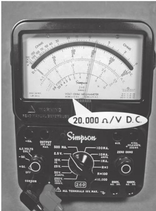
**Figure 1.23** Impedance specification for a typical analog meter.
