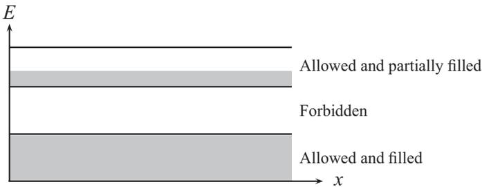
**Figure 3.2** Energy band structure for a conductor.
