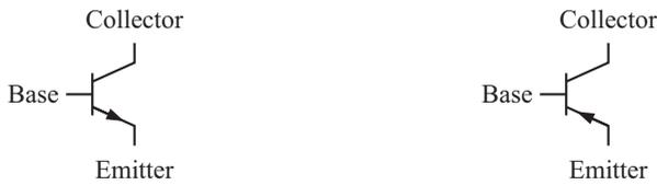
**Figure 4.1** Circuit symbols for the npn (left) and pnp (right) transistors.
