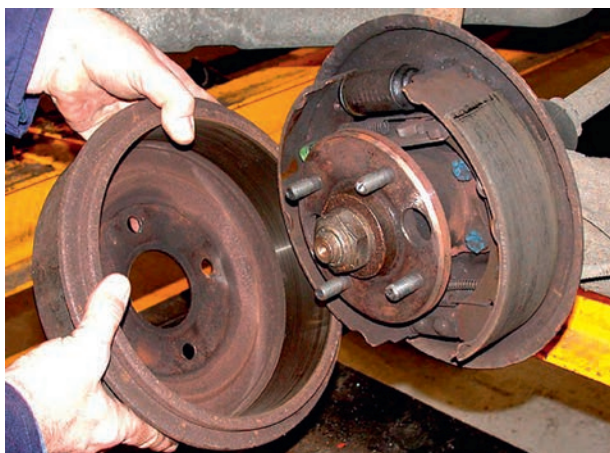
Figure 4.94 Brake drum being removed
