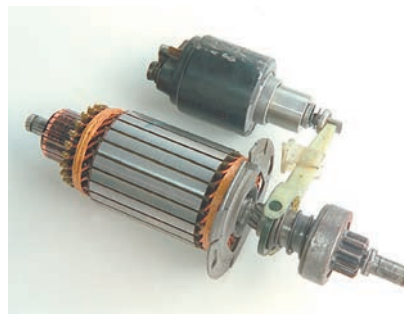
Figure 3.64 One-way clutch behind the drive pinion
