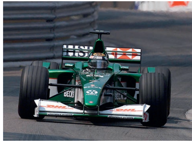
Figure 4.67 F1 cars use negative camber
