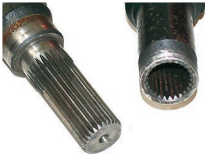
Figure 5.87 A splined joint connects to the gearbox
