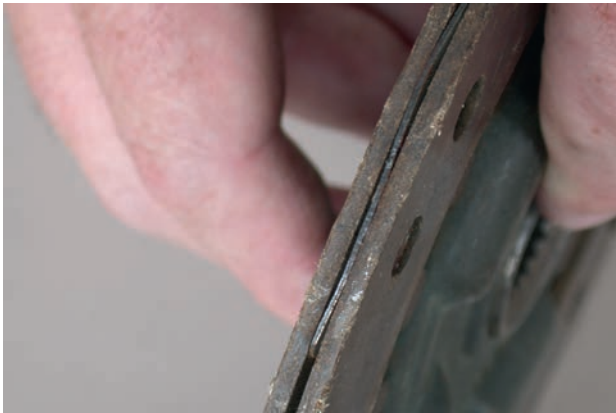
Figure 5.11 Wave springs eliminate chatter
