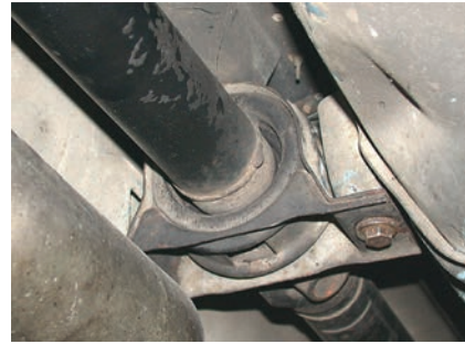
Figure 5.88 This rubber mounted bearing prevents propshaft whip
