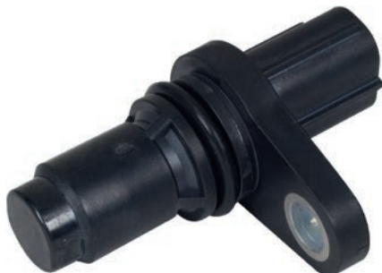
Figure 2.239 An inductive speed sensor produces a sine-wave signal, the frequency being proportional to engine speed. (Source: Denso Media)
