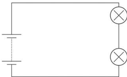
Figure 3.10 A simple series circuit
