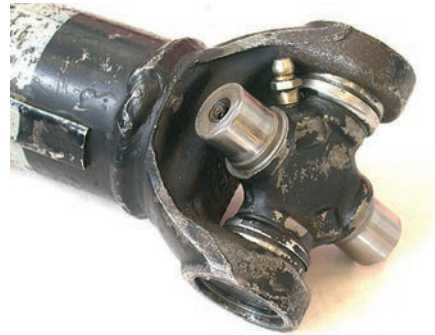
Figure 5.82 Detail of a universal joint
