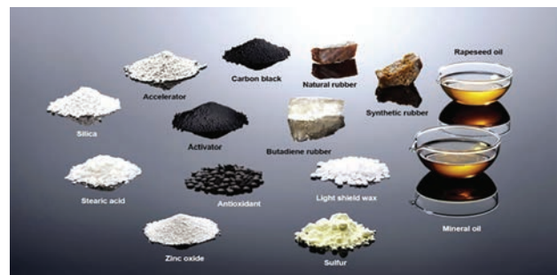
Figure 4.140 Overview of tyre materials. (Source: Continental)
