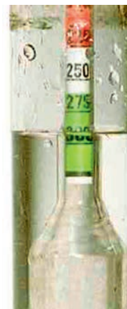
Figure 3.48 Reading a hydrometer: fully charged
