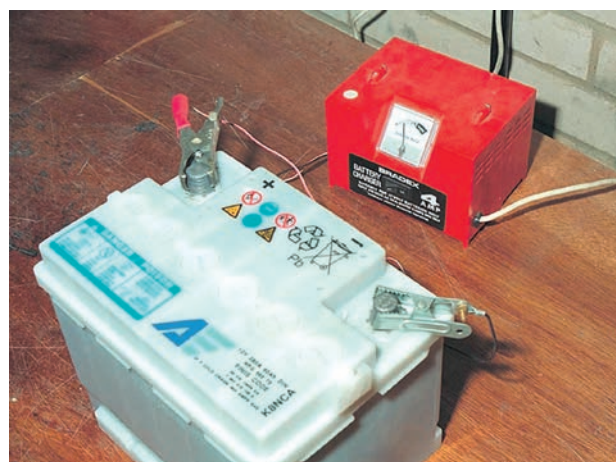
Figure 3.51 Recharging with a small bench charger
