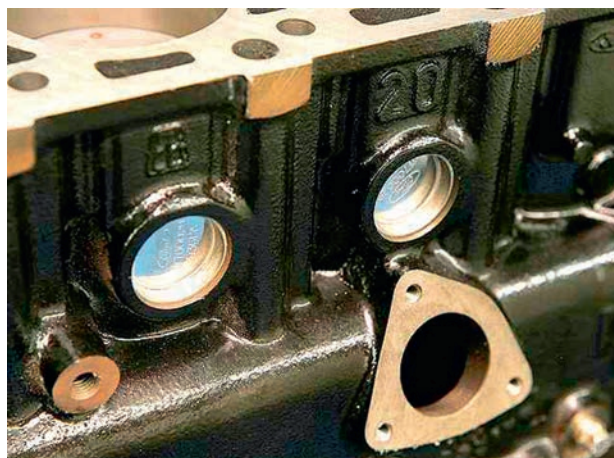
Figure 2.142 Engine block water jacket and core plugs
