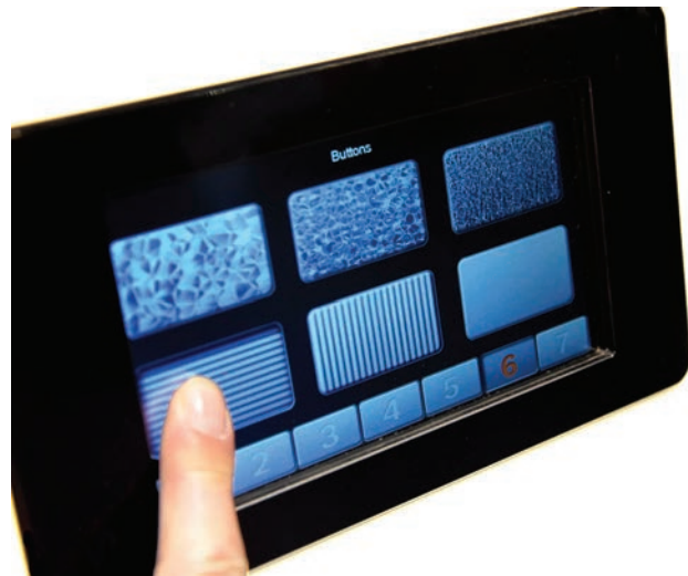
Figure 3.169 touchscreen with feedback. (Source: Bosch Media)
