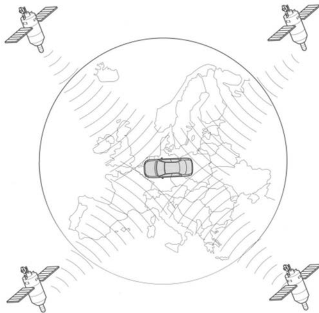
Figure 3.158 Four satellites determine vehicle position more accurately
