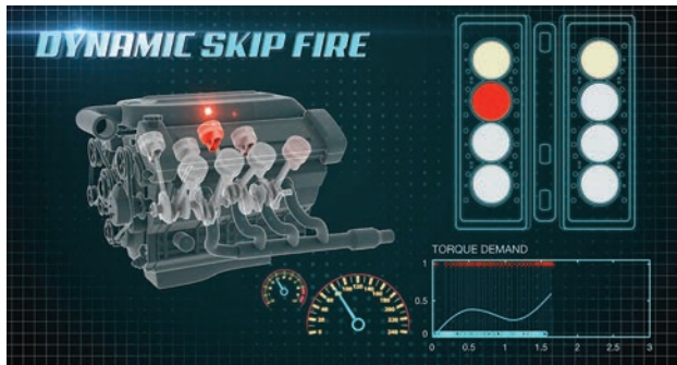
Figure 2.325 DSF Operation tracking engine torque demand. (Source: Tula, www.tulatech.com )
