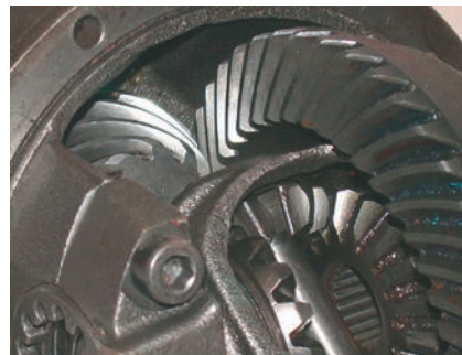
Figure 5.114 This differential is described as an open type
