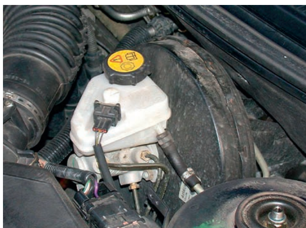
Figure 4.100 Master cylinder and fluid reservoir fitted on to the servo
