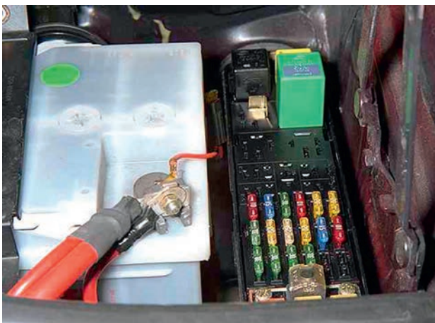
Figure 3.55 Correct polarity is important: red cables are used for the positive connection
