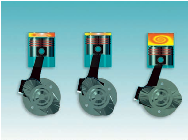
Figure 2.23 Ideal, retarded and advanced ignition point
