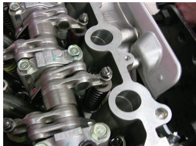
Figure 2.324 Honda cylinder deactivation mechanism
