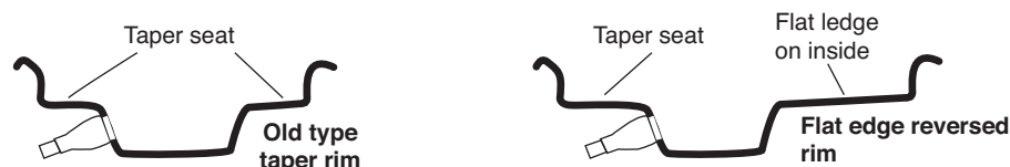
Figure 4.128 All car rims are well base. Early ones were intended for cross-ply, tubed type small section tyres, which were usually less than 5 inch rim width and a low flange height
