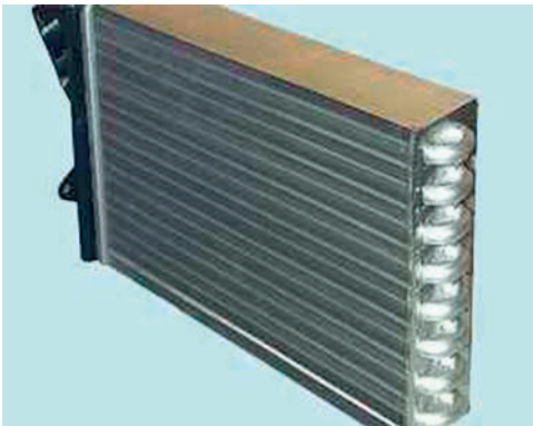
Figure 2.162 The heater matrix (radiator) is similar to the main radiator but smaller
