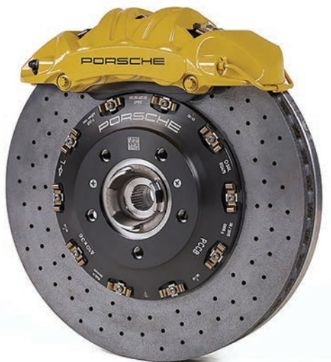
Figure 4.168 Since 2000, carbon ceramic has also been used in the production of braking systems for sports cars
