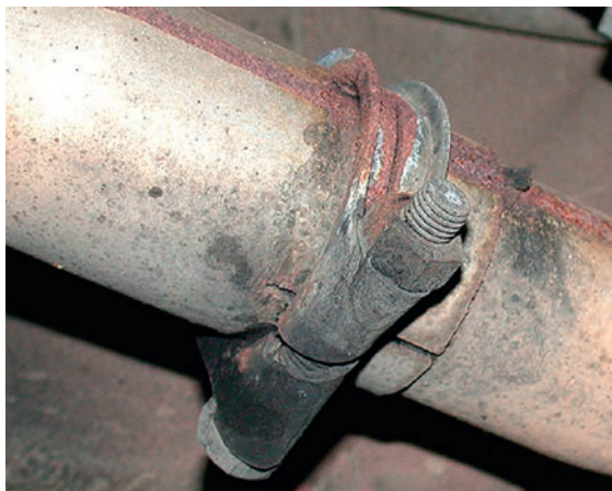
Figure 1.71 Corrosion on an exhaust joint
