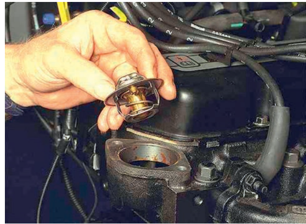
Figure 2.154 Thermostat with its wax pellet in the hot-coolant area
