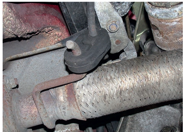
Figure 2.197 Flexible mountings (sometimes called pig noses)
