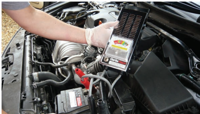
Figure 3.172 A high-rate discharge tester can indicate battery state-of-health, but still relies on the skill and judgement on the technician. In addition, there are several health and safety related issues to this approach! Note the tester in the picture is a fixed load, and not really suitable for the battery shown. (Source: www.autoexlex.co.uk )
