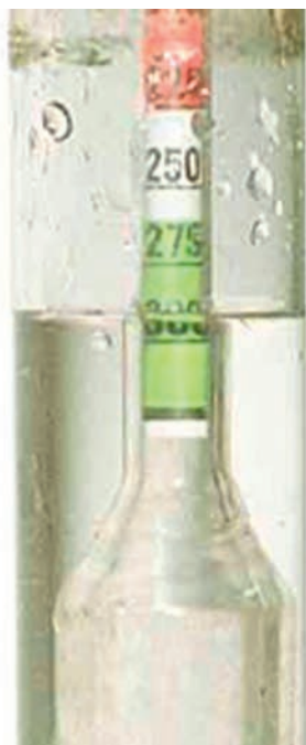
Figure 1.59 Measuring relative density with a hydrometer
