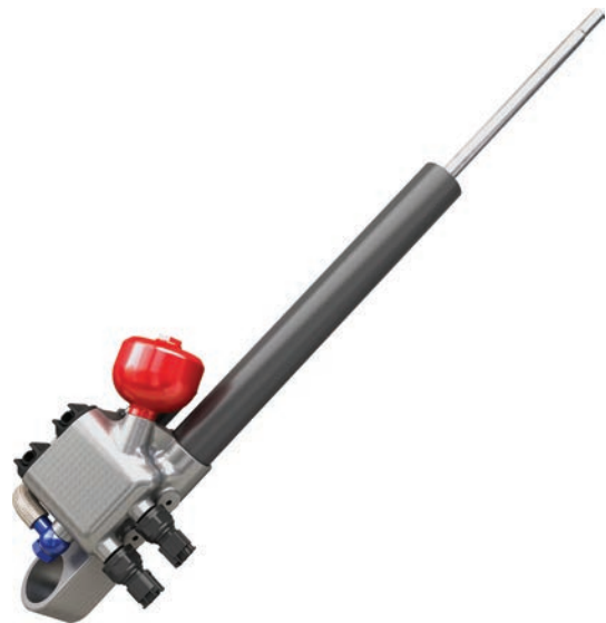
Figure 4.175 Damper for the active ride control system. (Source: Tenneco/Monroe ACOCAR)
