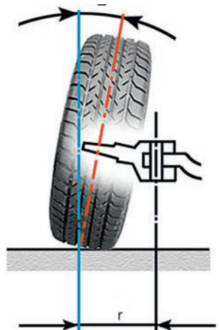
Figure 4.66 Negative camber ( r = scrub radius)
