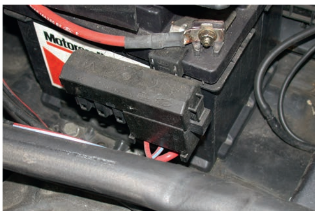
Figure 3.20 Heavy cable from the battery
