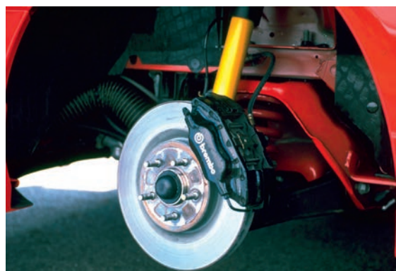
Figure 4.90 Flexible and metal brake pipes
