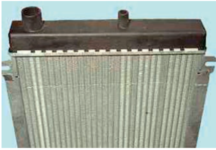
Figure 2.161 Aluminium and plastic radiator
