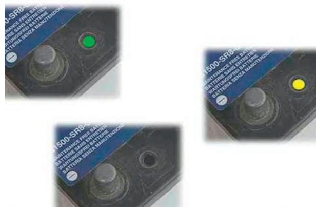
Figure 3.50 Maintenance-free battery hydrometer colours
