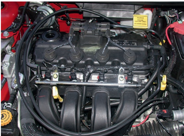
Figure 2.307 Distributorless ignition coil in position
