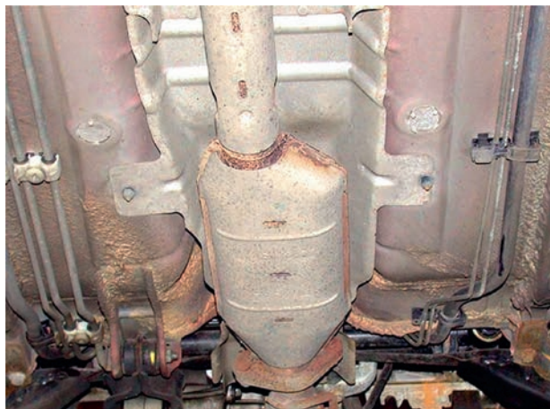
Figure 2.199 Catalytic converter in position with a heat shield above
