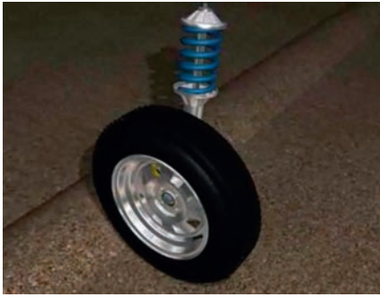
Figure 4.2 Spring just before a bump
