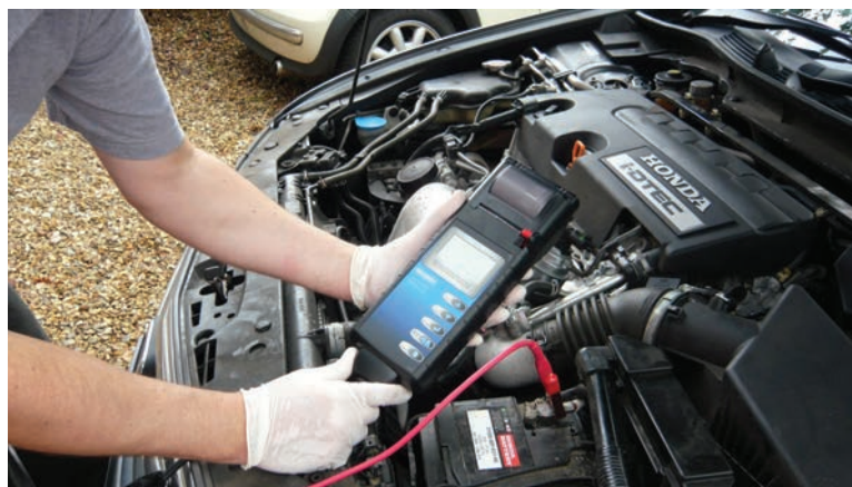
Figure 3.173 Intelligent, digital battery testers are much safer, and more appropriate for testing modern battery technology. (Source: www.autoelex.co.uk )
