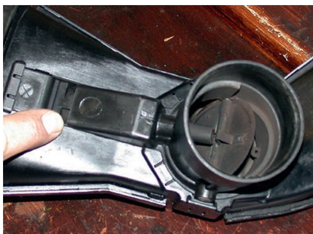
Figure 2.190 Warm-air control (vacuum type)
