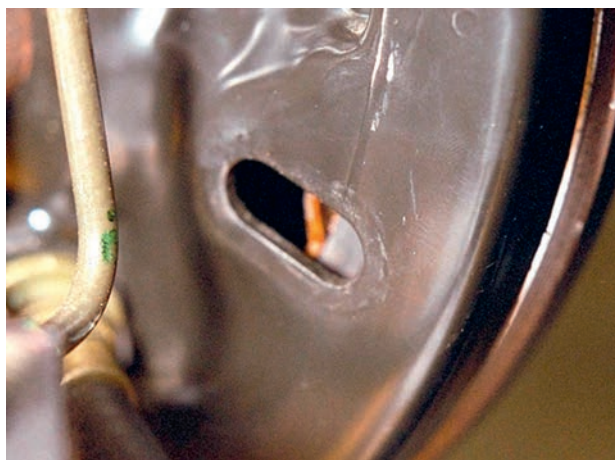
Figure 4.96 Drum brake adjustment hole
