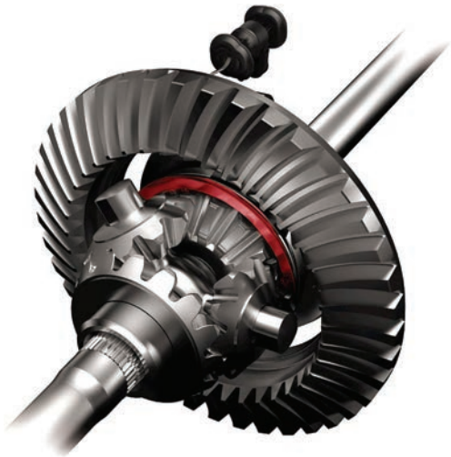
Figure 5.116 Differential locking mechanism [highlighted]. (Source: Ford Media)
