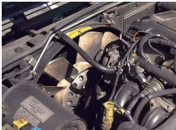
Figure 2.169 Viscous-fan hub on an earlier engine
