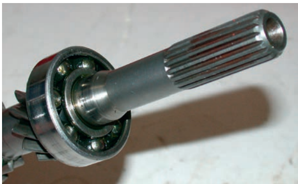
Figure 1.95 This bearing on a gearbox shaft is held in place by compression
