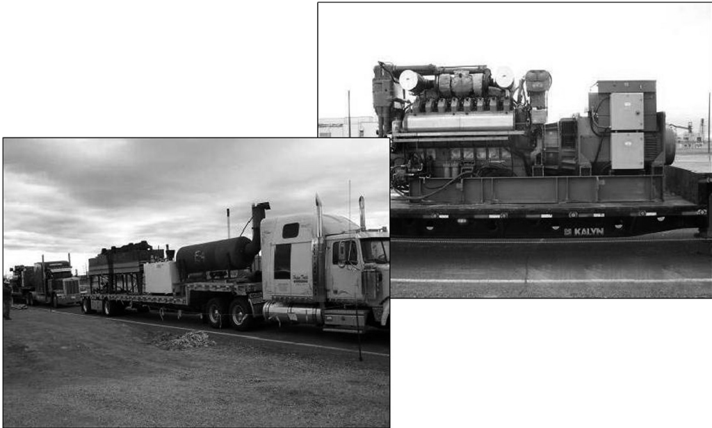
Figure 6.4 Generator used for the Aurora generator test. ( https://muckrock.s3.amazonaws.com/foia_files/14f00304-Documents.pdf , p. 103.)
