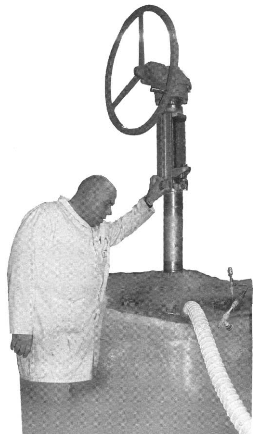
Figure 3.54 Cryogenic valve testing Courtesy of YPS Valves Ltd
