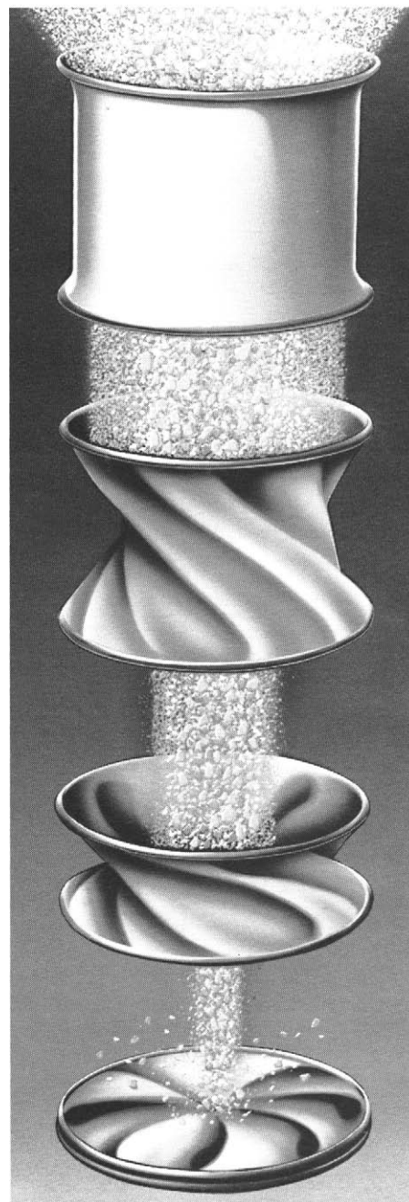
Figure 3.88 Operation of the iris diaphragm valve Courtesy of Kemutec Powder Technologies Ltd
