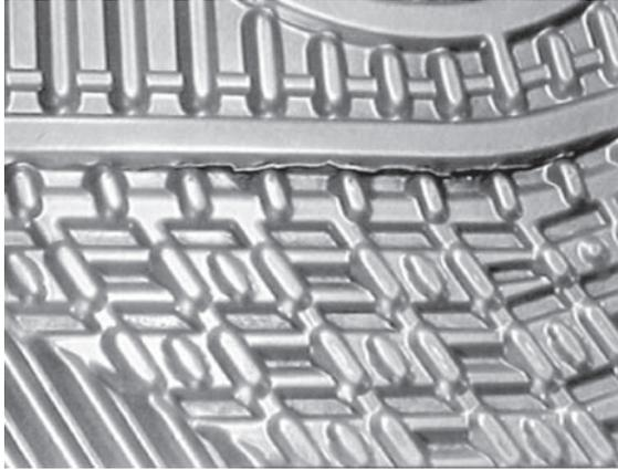
Figure 9.15: Corrosion fatigue of plates [31].
