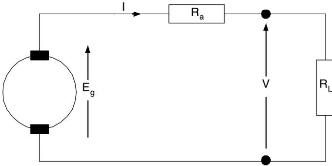
**Figure 4.9.** The equivalent circuit of a brushed tachogenerator.
