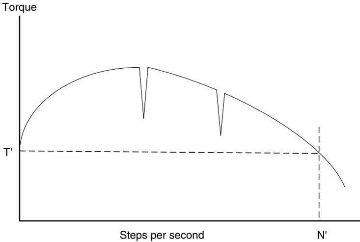
**Figure 8.6.** Typical pull-out torque-speed characteristics of a stepper motor: the dips in the curve are resonance points. In order to achieve torque throughout the speed range, a value less than the peak torque must be selected.
