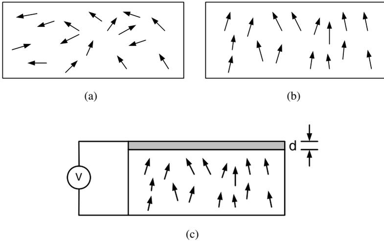
**Figure 9.5.** The characteristic of a piezoelectric material. (a) shows domains in the unpolarised material, which align when polarised, as shown in (b). The application of a voltage causes axial displacement,  $d$ .
