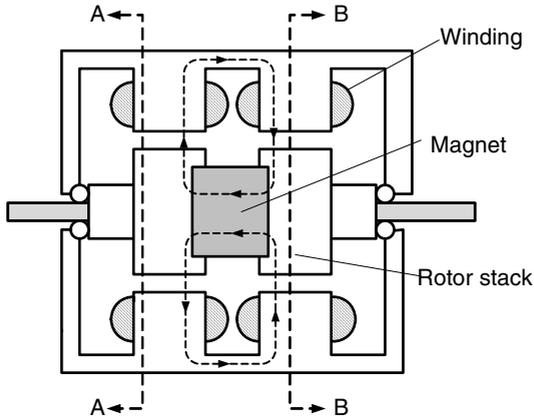
(a) Longitudinal cross section through the motor.
