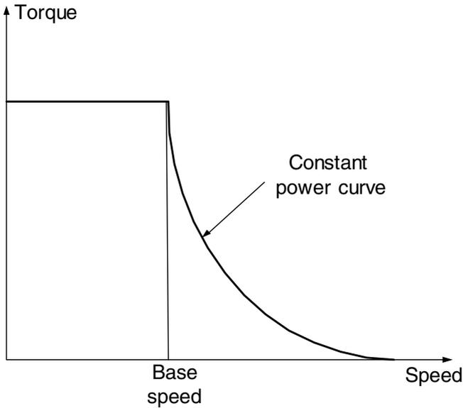
**Figure 6.10.** The torque speed characteristics of a sinewave wound machine. Above base speed  $\beta$  can be adjusted to increase motor speed, however a constant power limit as defined by equation (6.31) will apply.
