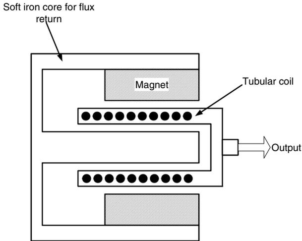
**Figure 9.1.** The cross section of a voice coil; the dimensions of the air gap has been exaggerated.
