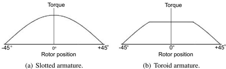
**Figure 9.3.** Torque-position characteristics for a limited angle torque motor.
