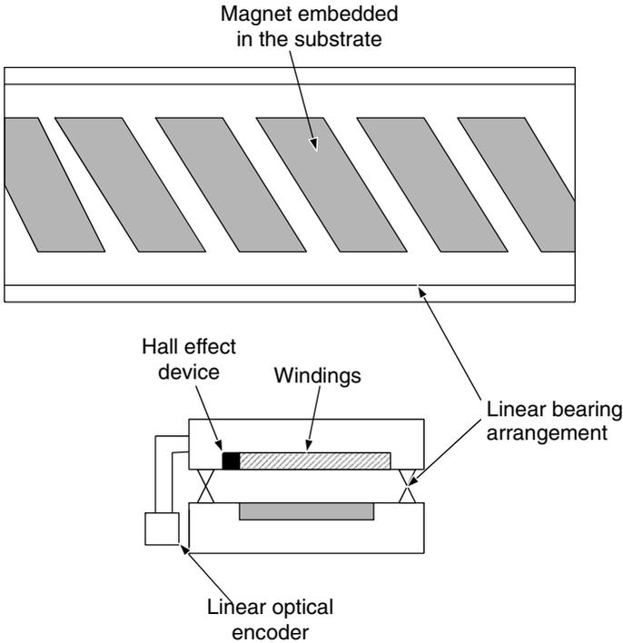
**Figure 6.12.** The construction of a linear brushless motor. The upper figure shows the plan of the substrate, the lower shows a cross section through the substrate and the carriage that contains the windings.
