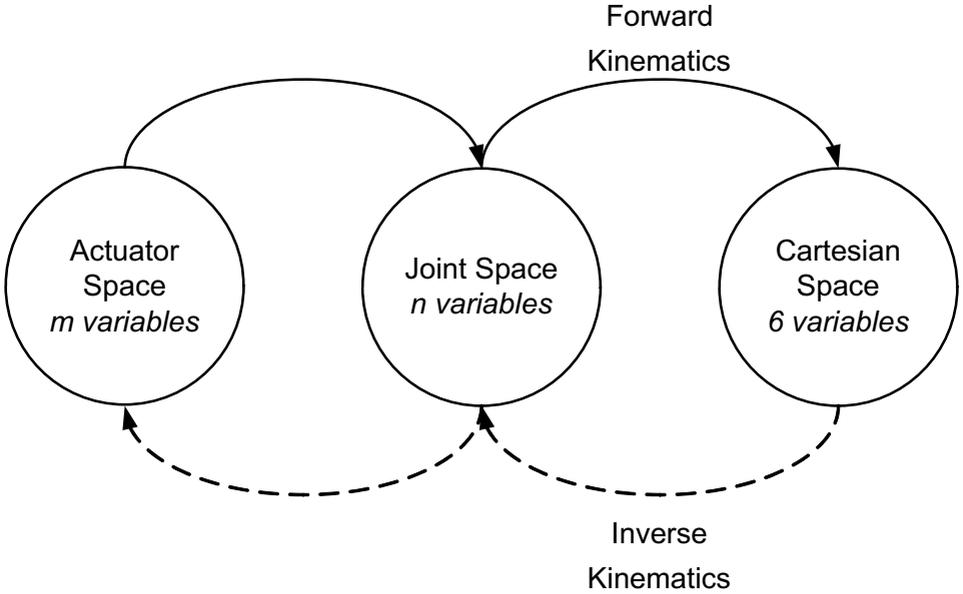
**Figure 1.7.** The mapping between the kinematic descriptions. The number of variables in Cartesian space is 6, while the number of variables in joint and actuator space is determined by the manipulators's design.
