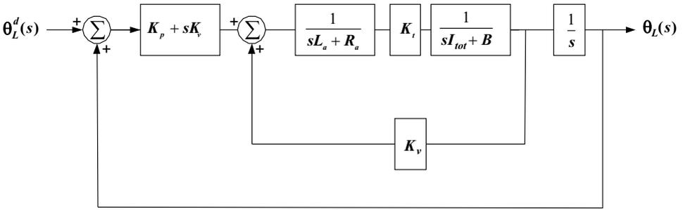
**Figure 10.2.** The block diagram for a closed-loop controller.
