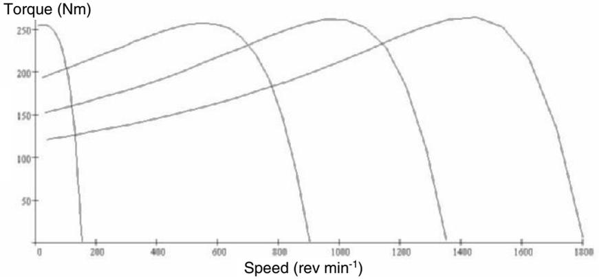
**Figure 7.7.** Torque-speed characteristics of the motor for supply frequencies of 5, 15, 30, 45 and 60 Hz. The supply voltage has been controlled to maintain constant. It should be noted that to give maximum torque at standstill, the supply frequency needs to be approximately 5 Hz.
