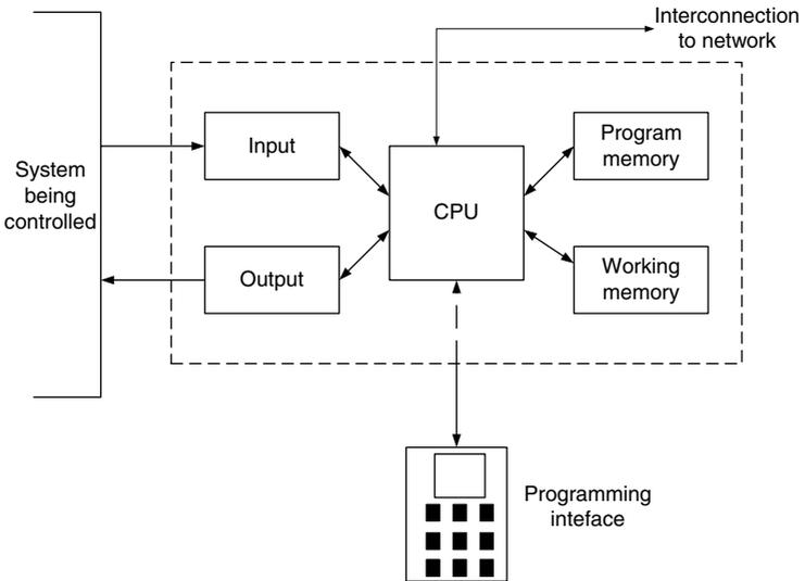
**Figure 10.10.** The internal structure of a PLC.
