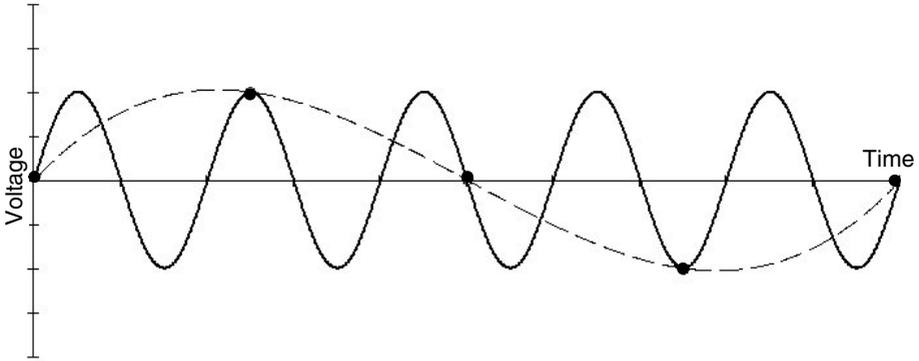
**Figure 4.6.** Aliasing caused by a sampling frequency. The sampling points are shown as dots, the sampling frequency is below the frequency of the waveform being sampled. The reconstructed waveform is shown as the dotted line.
