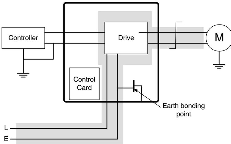
**Figure 2.11.** A possible wiring layout for a drive system in a normal industrial environment. The motor cables are twisted to reduce interference, the cabinet is provided with a bonding point. While the controller is separately earthed, care needs to be taken to prevent earth loops. In order to prevent problems, any sensitive electronics should be placed a distance away from various elements as shown by the shaded areas.
