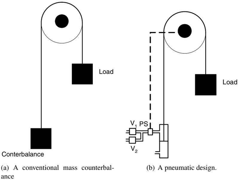
**Figure 2.10.** The use of a counterbalance to reduce the motor's continuous loading in a vertical drive application. In the pneumatic design the valves  $V_1$  and  $V_2$  ensure that the pressure difference in the cylinder remains constant; if the air pressure is lost a low pressure switch activates a brake.
