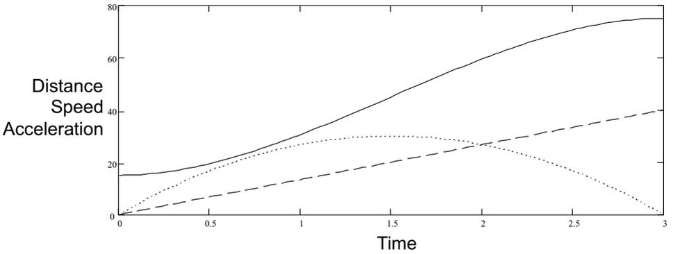
**Figure 2.9.** Position, velocity and acceleration profiles for a single cubic segment where  $\theta_1 = 15^\circ$ ,  $\theta_2 = 75^\circ$ , the move time is given by  $t_m = 3$  s, at the start and end positions the system is at rest. The distance moved is shown as a solid line, the speed as dotted and the acceleration as dashed.
