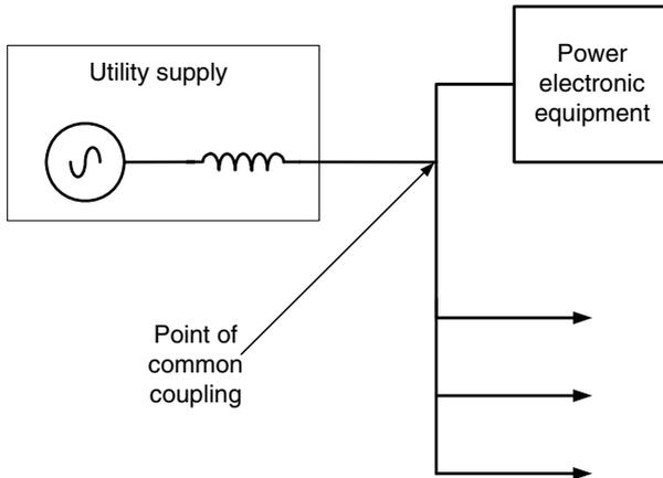
**Figure 2.13.** The utility interface, showing the *point of common coupling*, where the supply distortion caused by each individual load is combined, due to the finite impedance of the supply – here represented by a simple inductance.
