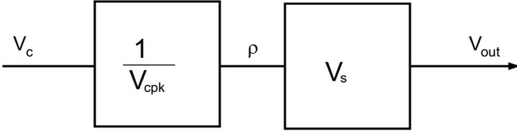
**Figure 5.11.** The equivalent circuit of a PWM amplifier.
