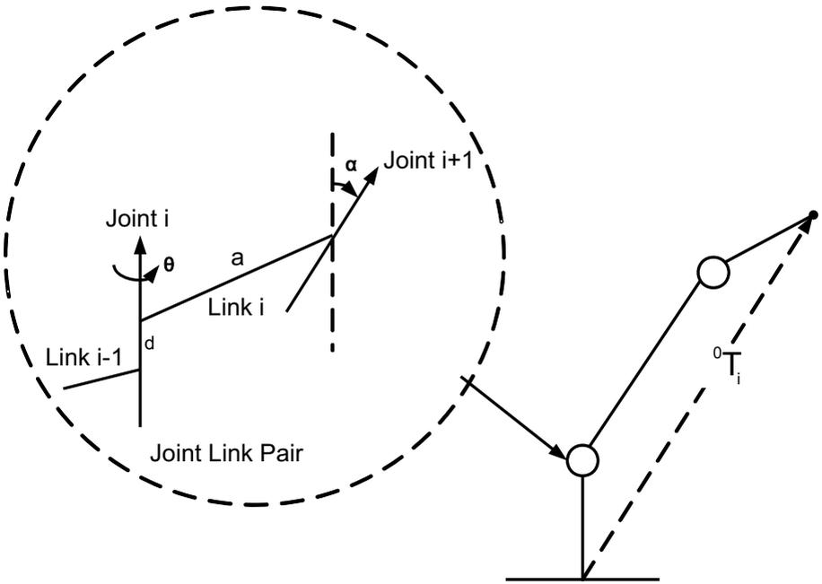
**Figure 1.6.** Joint-transformation relationships for a robotic manipulator.
