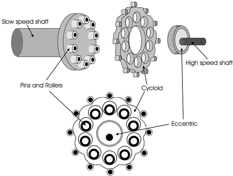
**Figure 3.5.** A schematic diagram of a cycloid speed reducer. The relationship between the eccentric, cycloid and slow-speed output shaft is clearly visible. It should be noted that in the diagram only one cycloid disc is shown, commercial systems typically have a number of discs, to improve power handling.
