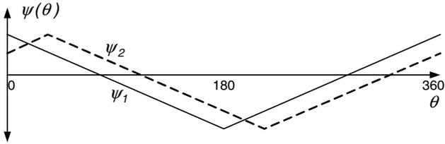
(b) The magnetic flux linkage in the airgap,  $\psi(\theta)$
