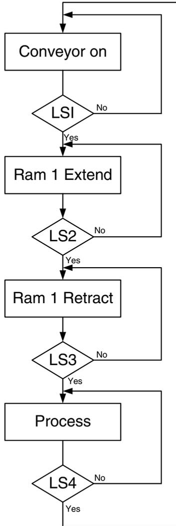
**Figure 10.16.** The flowchart for the process line.
