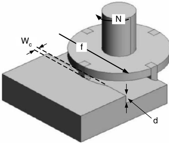
**Figure 1.3.** The face-milling process where the workpiece is being reduced by  $d$ :  $f$  is the feed rate of the cutter across the workpiece,  $W_c$  is the depth of the cut and  $N$  is the rotary speed of the cutting head.
