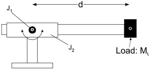
**Figure 2.5.** The effective load inertia of a rotary joint,  $J_1$ , changes as the linear joint,  $J_2$  of polar robot extends or retracts (the YY axis of the joint and the load point out of the page).
