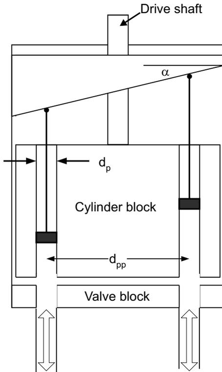
**Figure 1.16.** The displacement hydraulic pump used in an EHA. Driving the valve cylinder causes the pistons to operate, the amount of stroke is determined either by the rotation speed, or the swash plate angle,  $\alpha$ . The clearances between the cylinder block and, the valve block and casing have been exaggerated.
