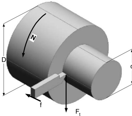
**Figure 1.2.** The turning process, where a workpiece of initial diameter  $D$  is being reduced to  $d$ ;  $F_t$  is the tangential cutting force,  $N$  is the spindle speed, and  $f$  the feed rate. In the diagram the depth of the cut is exaggerated.
