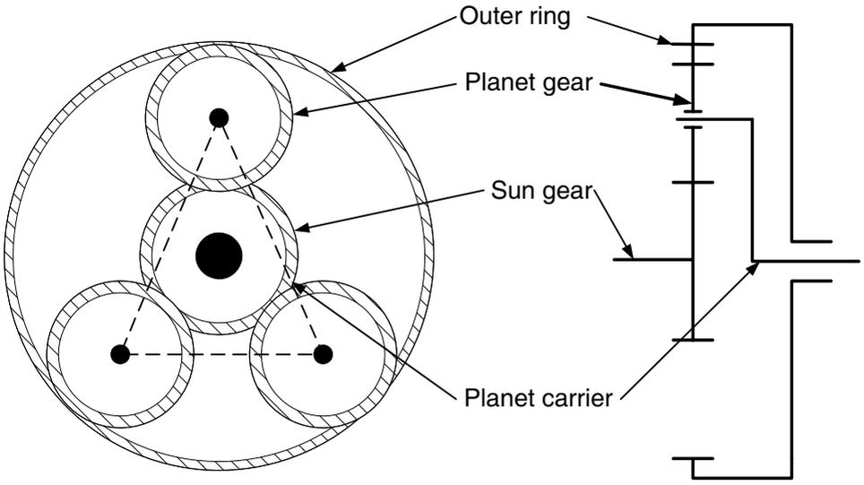
**Figure 3.3.** A planetary gearbox; the output from the gearbox is from the three planet gears via the planet carrier, while the sun gear is driven. In this case the outer ring is fixed, the input is via the sun, and the output via the planet carrier.
