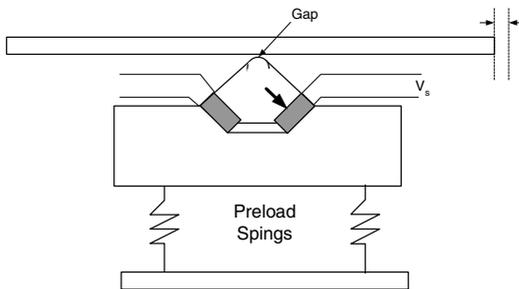
(c) Excitation of the piezoelectric material ( $V_s < 0$ ), releases the actuator from the wear surface, allowing the actuator to return to its initial position.
