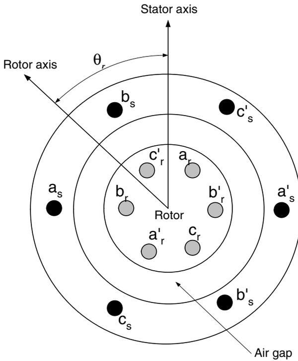
**Figure 7.1.** Cross section of an idealised three-phase, two-pole induction motor. The rotor and stator windings are represented as concentrated coils. The rotor's speed is  $\omega_r$ , and the lag between the rotor and stator axes is  $\theta_r$ .
