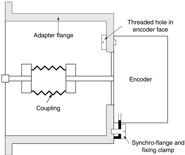
**Figure 4.21.** Connecting an encoder to a shaft using a bellow coupling and adapter flange. Threaded holes can be provided on the face of the encoder, or if the encoder is fitted with a synchro-flange, fixing clamps can be used.
