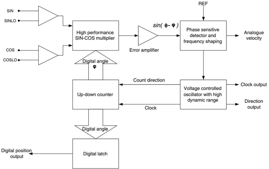
**Figure 4.14.** Internal function block diagram of a resolver-to-converter. The two stationary windings of the resolver are connected to SIN and SINLO, and COS and COSLO respectively. The resolver is powered by an external oscillator, which also provides the REF signal.
