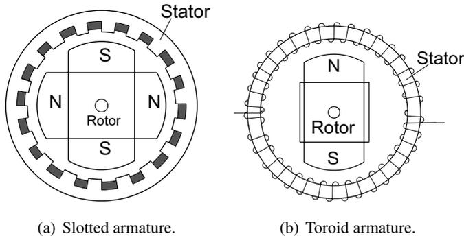
**Figure 9.2.** Internal construction of limited angle torque motors.
