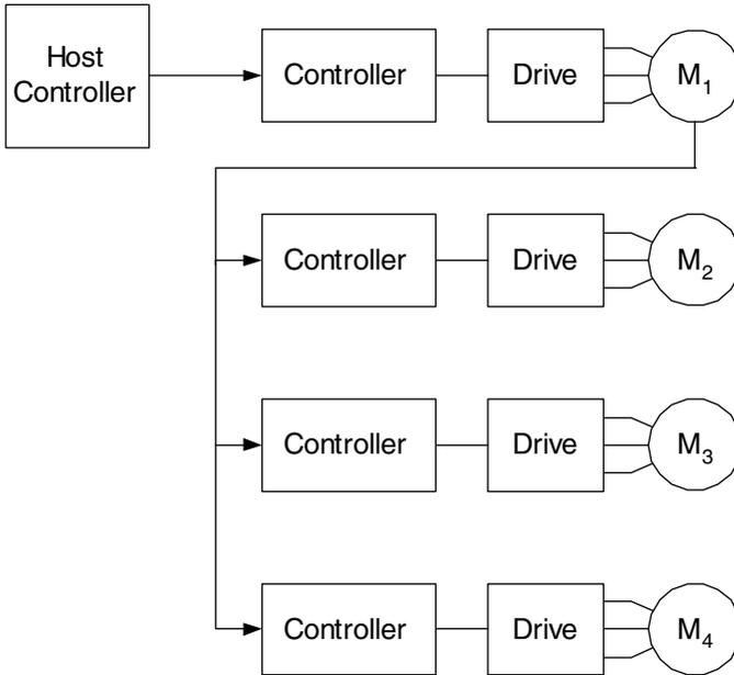
**Figure 10.7.** The use of a number of single-axis controllers to provide an electronic line shaft. The motors  $M_2$  to  $M_4$  operate with a fixed positional relationship to  $M_1$ . The relationship is determined by the individual axis parameters.
