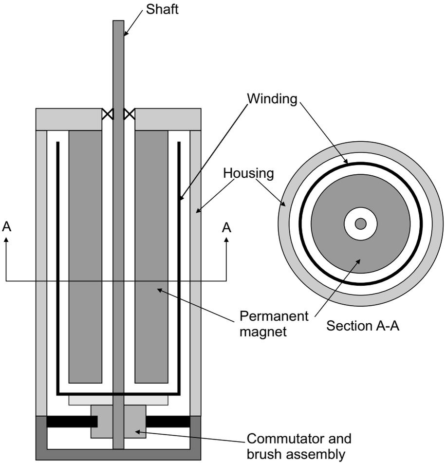
**Figure 5.2.** The construction of an ironless-rotor motor.
