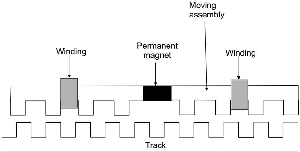
**Figure 8.4.** Cross section of a linear stepper motor. The motor consists of a stationary track, and a moving assembly incorporating magnets and the windings. As shown in the diagram, only one set of teeth on the moving assembly aligns with the track teeth.
