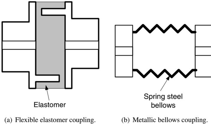
**Figure 3.12.** Cross sections of commonly used couplings.
