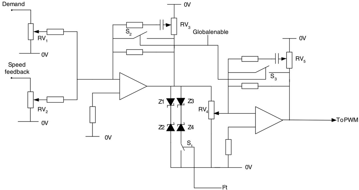
**Figure 5.17.** Details of an analogue stage for a PWM amplifier suitable for d.c. motor control. The CMOS analogue switches are used to control the  $I^2t$  limit ( $S_1$ ) and the amplifier disables ( $S_2$ ) and ( $S_3$ ). The peak current is set by  $Z_1$  and  $Z_2$ , with the  $I^2t$  foldback limit set by  $Z_3$  and  $Z_4$ .
