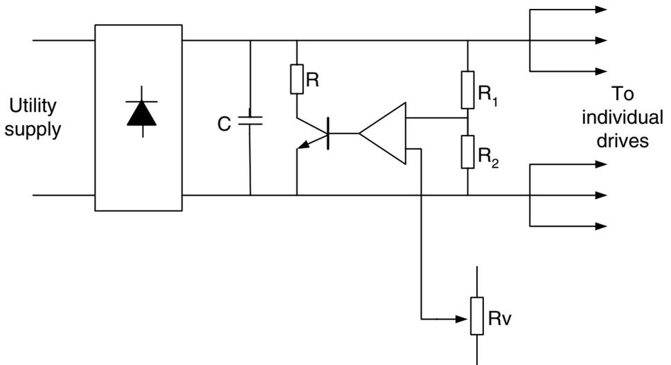
**Figure 5.21.** A single phase power supply for a drive system, including a shunt voltage regulator. The switching voltage is determined by the variable resistor,  $R_v$ . The shunt resistor is identified as  $R$ .
