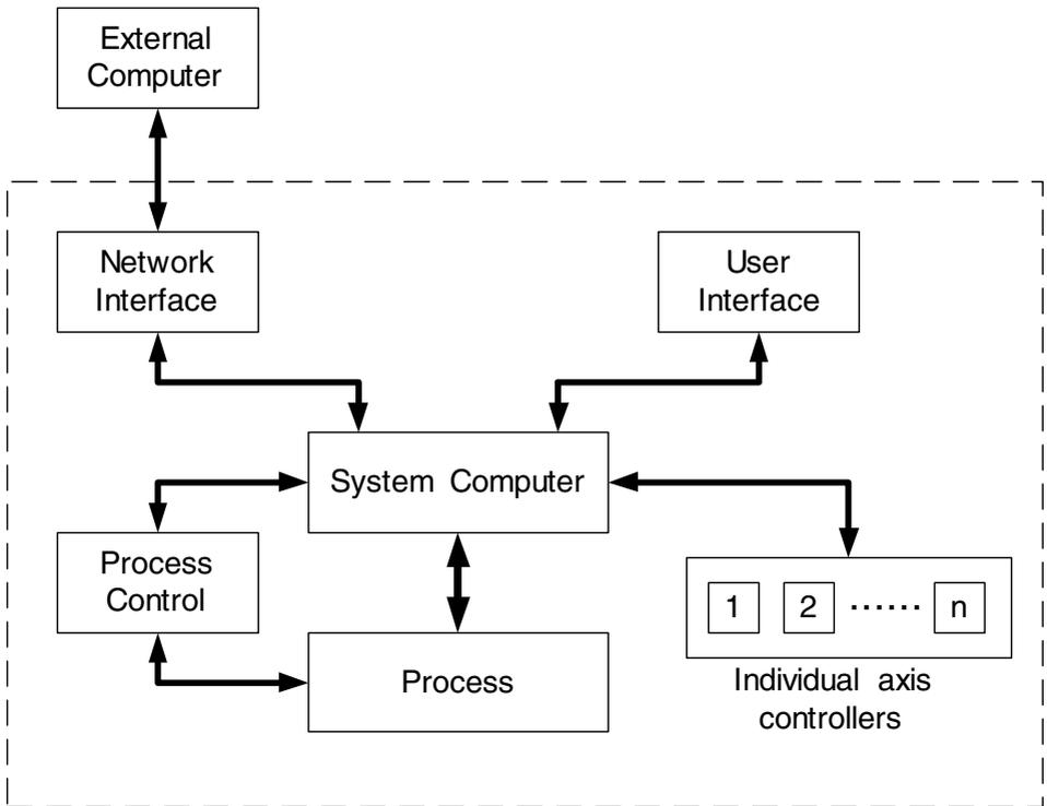
**Figure 1.1.** The outline of the control structure for CNC machine tool, robot or similar multi-axis system. The number of individual motion axes, and the interface to the process are determined by the system’s functionality.
