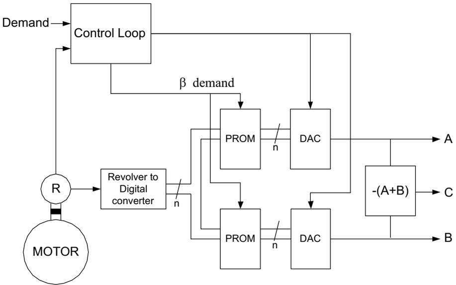
**Figure 6.11.** The block diagrams of a sinewave wound machine controller, using a resolver as the position transducer. The control loop provides two signal, an analogue input to the multiplying DACs and  $\beta$  as digital word to the PROMs to allow operation above base speed. The three outputs (A,B and C) are fed via a suitable power amplifier to the motor.
