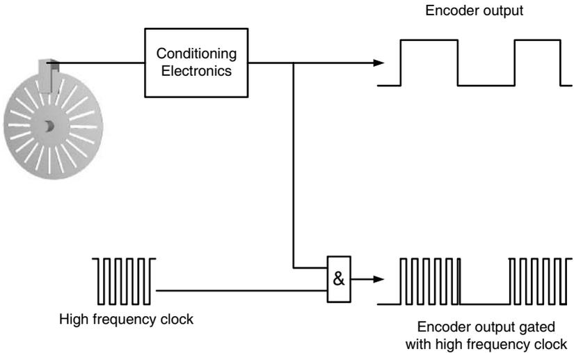
**Figure 4.10.** Speed-measurement using an incremental encoder. The output can be directly taken from the conditioning electronics, or to increase the resolution, the encoder waveform can be gated by a high frequency carrier.
