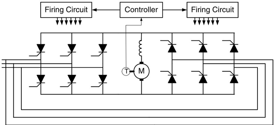
**Figure 5.6.** A four quadrant thyristor drive for d.c. brushed motors. This system as shown is not capable of handling circulating currents. To prevent circulating current the supplies must be isolated from each other through the use of a transformer.
