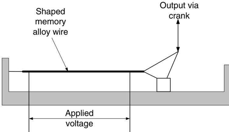
**Figure 9.10.** The use of a shaped-metal-alloy wire as part of an actuator. The voltage across the wire, and the current through the wire which gives rise to wire heating, is from the output of a conventional position control loop.
