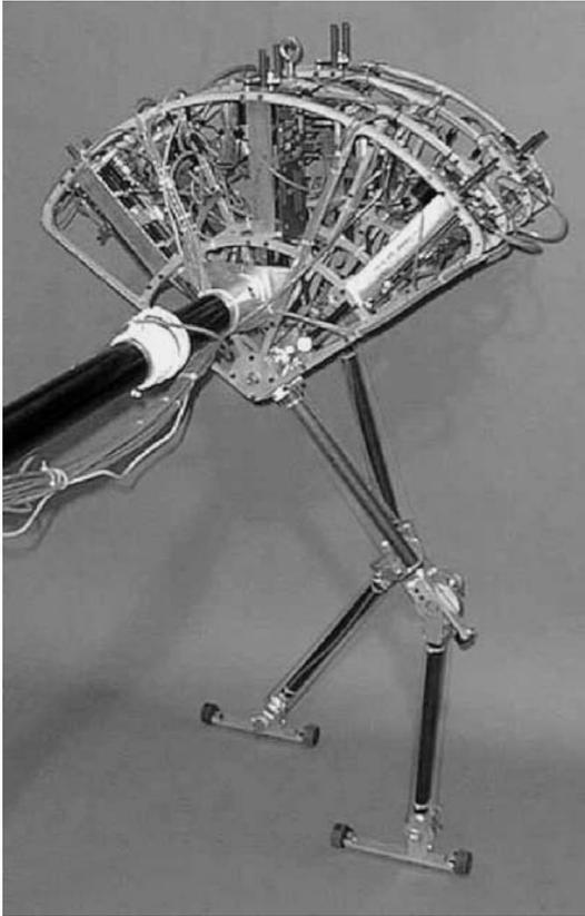
**Figure 1.12.** Spring Flamingo, a 6 degree-of-freedom planar biped robot, was developed at the MIT Leg Laboratory. Spring Flamingo is capable of human-like walking at speeds of up to  $1.25 \text{ m s}^{-1}$ . Picture reproduce with permission from Jerry Pratt, Yobotics, Cincinnati, OH.
