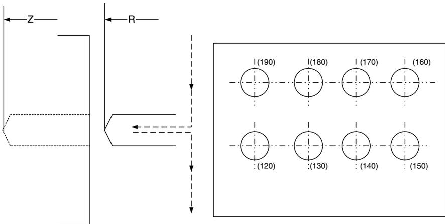
**Figure 10.8.** A drilling cycle using the canned cycle, G81. The cycle advances the drill to position R, and then feeds at drill speed to Z, and then retracts back to R. The controller then moves the drill to the next whole position, prior to the drilling being repeated. The numbers in brackets refer to the programme line responsible for drilling the hole.
