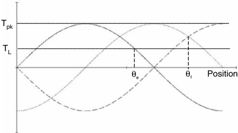
**Figure 8.9.** The static-torque characteristic for a stepper motor with an applied load. When a phase is energised the motor has to move from  $\theta_e$  to  $\theta_f$  without loss of synchronism. The three curves are the individual static-torque characteristics of the individual phases.
