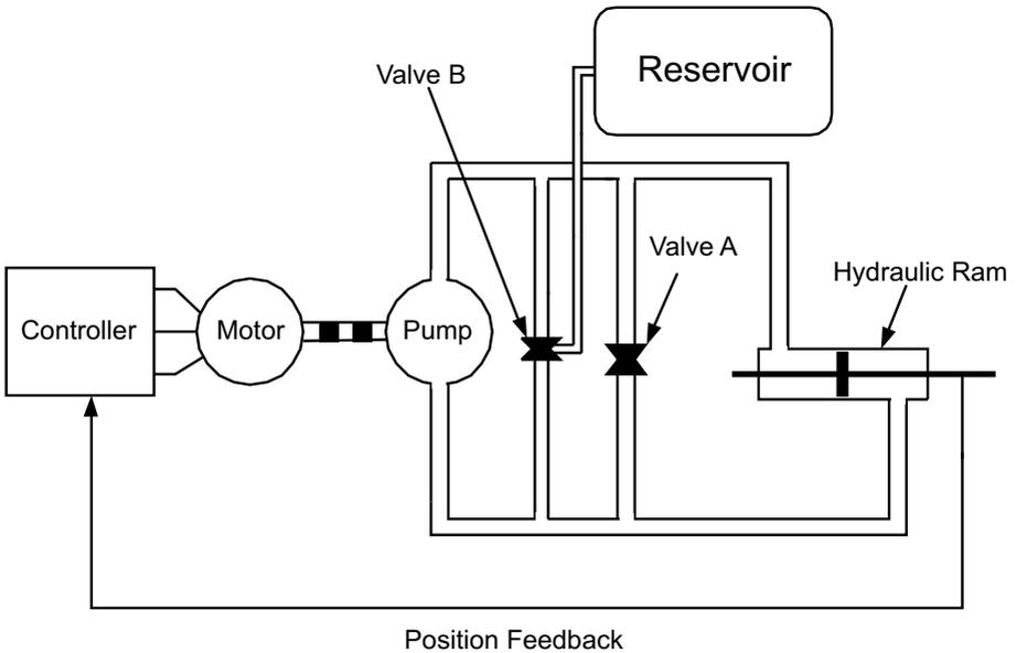
**Figure 1.17.** Concept of an electrohydrostatic Actuator for use in an aircraft. Value A is a bypass valve that can allow the ram to move under external forces in the case of a failure, while valve B ensures that the pressure of the input side of the pump does not go below that of the reservoir.
