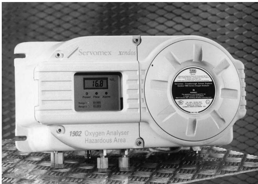
Figure 25.8 Example of a mixed concept apparatus which aids routine maintenance and adjustment. The circular threaded cover allows entry to a flameproof chamber and so must only be opened when de-energised, and under any other specific conditions which might be stated on the unit or in the associated documentation. The chamber contains only intrinsically safe circuits, thus permitting it to be opened at any time to allow access to, and live adjustment of, calibration or alarm setting controls, but subject of course to any extra operational conditions laid down by the manufacturer. Photograph courtesy of Servomex Group Ltd
