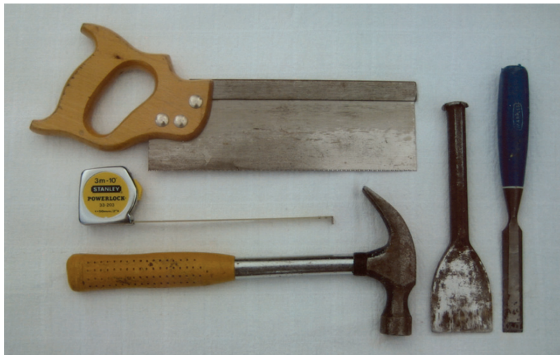
Figure 5.18 Some additional tools required by an electrician engaged in house wiring.
