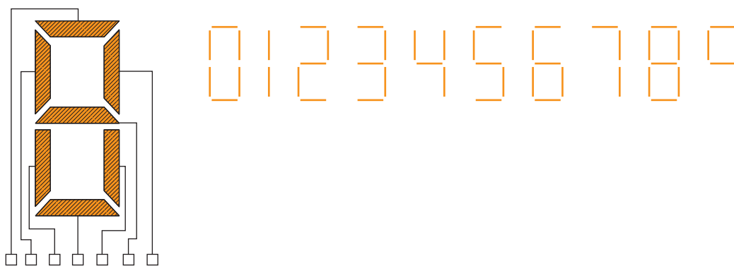
Figure 9.84 LED used in seven-segment display.
