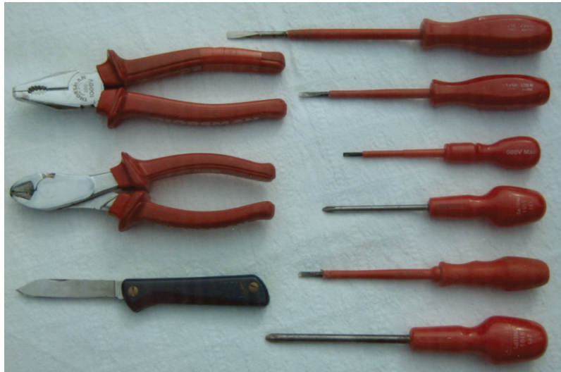
Figure 5.17 The tools used for making electrical connections.
